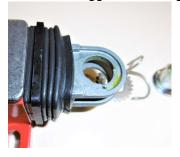
7) Remove the bellows from its anchorage, then from the truck Be careful the ring has a mounting orientation to lock the bellows
