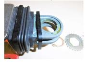
6) Unlock the biggest anchorage ring like shown on the picture
