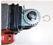
2) Remove the ratchet-locking→ the truck axis can be removed
